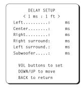
This menu, which is reached from the MAIN menu, allows you to set the delay time for each individual speaker. This is an important feature as it enables the sound from each speaker to arrive at the listening position at the same time, even when they are not all placed at equal distances from the listener. This preserves accurate sound imaging even with irregular speaker placements.
